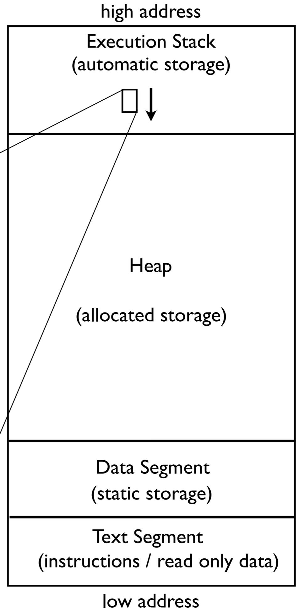
(\* ) *The C standard does not dictate any particular memory layout, so what is presented here is just a useful conceptual example model that is similar to what some architecture and run-time environments look like*
