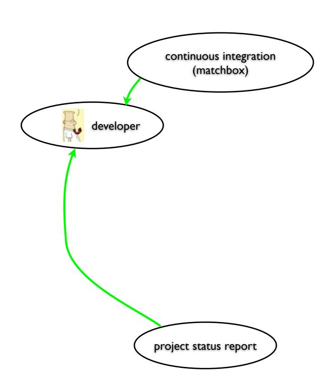
Any change applied to the shared codebase is immediately picked up by matchbox, our continuous integration system. Matchbox builds all products depending on that change, perhaps as many as ten products using different compilers targeting various processors.
