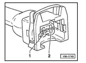
Check for open circuit and short to positive or Ground in following wiring connection:
