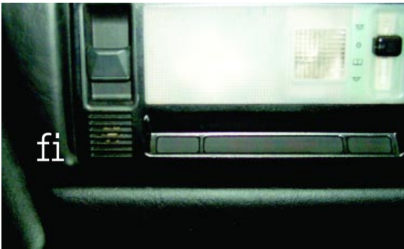
At the lower left corner of the courtesy/dome light is a small grille behind which is the cabin temperature sensor. A tube from it leads behind the passenger side outlet duct, where a small air pump constantly draws fresh air through the tube and over the sensor.
