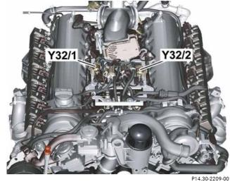
Y32/1 Air pump 1 switchover valve Y32/2 Air pump 2 switchover valve
