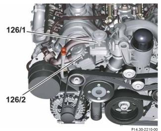
126/1 Left air shutoff valve 126/2 Right air shutoff valve
