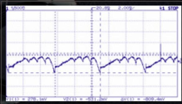
*An open diode may produce a pattern like this on a lab scope.*
