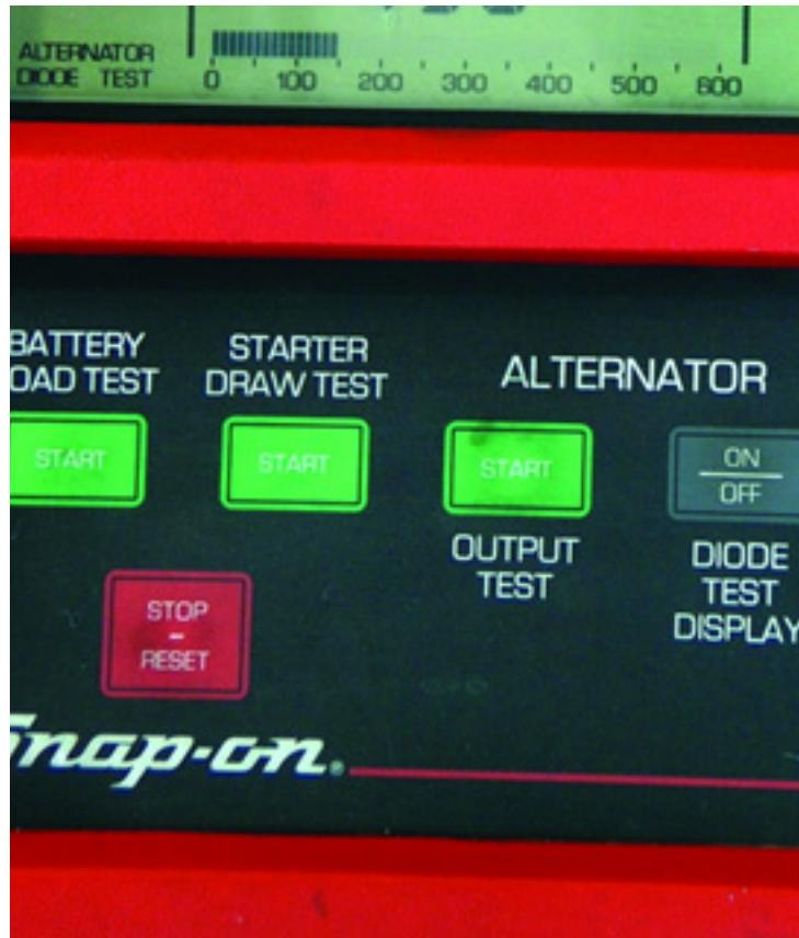
*Most VATs include a ripple function. This one reads out the actual AC content instead of just turning on a warning lamp.*
