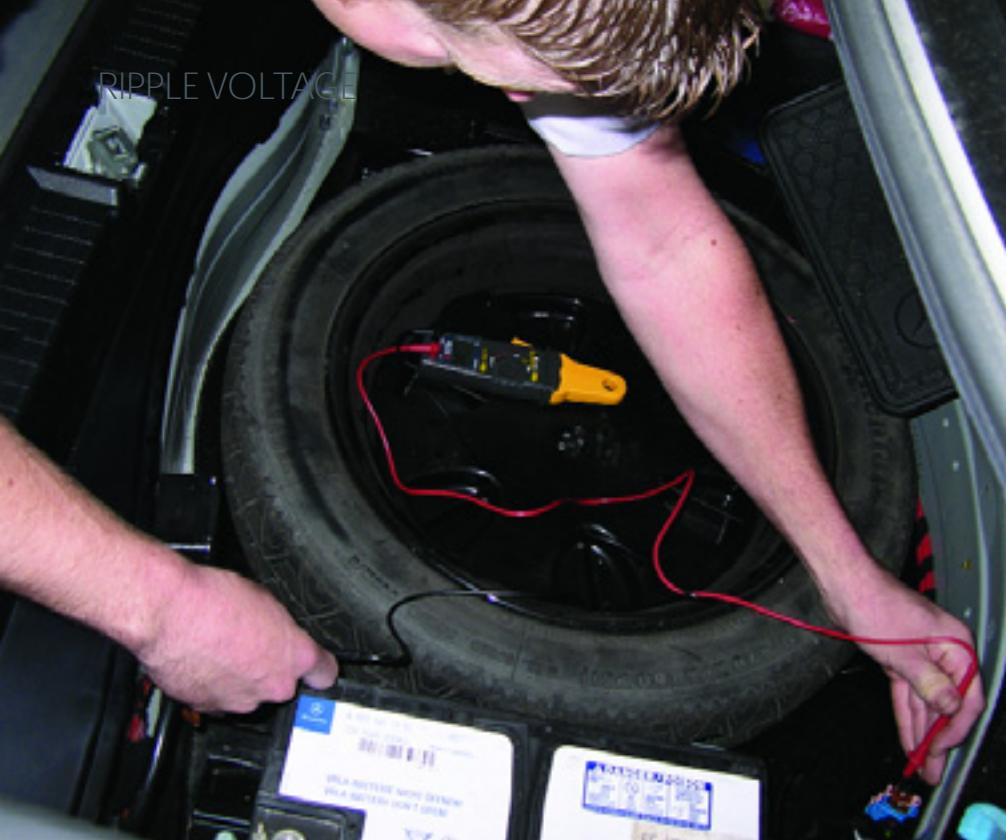
*A measurement of ripple at the battery terminals won't be as accurate as taking it at the alternator.*
