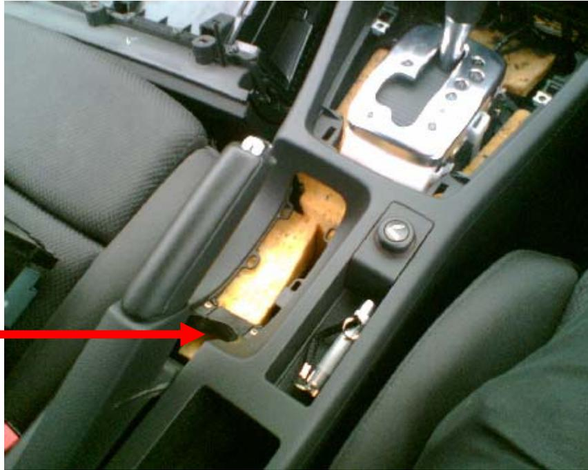
Picture of the Centre Console after it has been removed.
