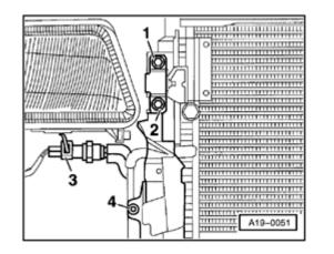
Unbolt pressurizing fan and detach cooling lines for power steering hydraulic fluid -arrows-.
