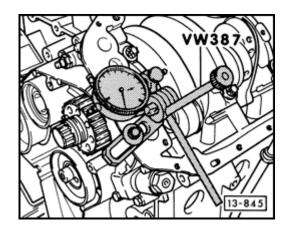
Crankshaft axial and radial clearance, checking
