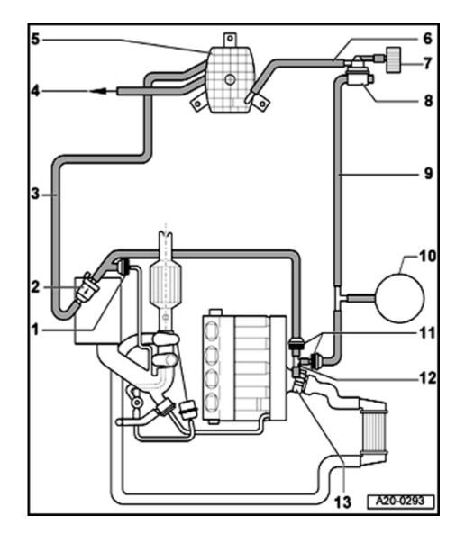
EVAP system leak detection circuit, schematic diagram (vehicles with 1.8 ltr. turbo engine)
