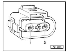
Check the following wire connection for open circuit and short circuit to Ground (GND) or to plus (B+):
