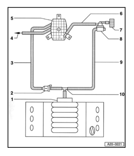
EVAP system leak detection circuit, schematic diagram (vehicles with 2.8 ltr. engine)
