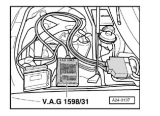
Connect test box VAG1598/22 to harness connector. The ground clamp (not visible in the illustration) must be connected to battery ground connection. Do not connect ECM.
