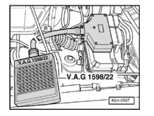
Connect test box VAG1598/22 to harness connector. Do not connect ECM.
