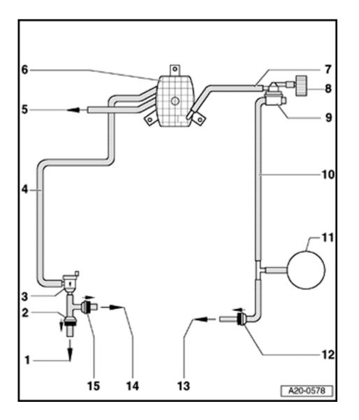
EVAP system leak detection circuit, schematic diagram (vehicles with 2.7 ltr. turbo engine)
