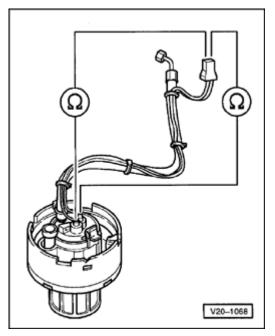
Check wiring between flange and fuel pump for continuity.
