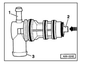
Fig. 1 Bleed valve, removing, installing, checking
